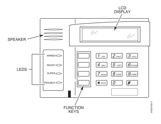
**IMPORTANT!** When using the keypad to enter codes and commands, sequential key depressions must be made within 3 seconds of one another. If 3 seconds elapses without a key depression, the entry is aborted and must be repeated from its beginning.
